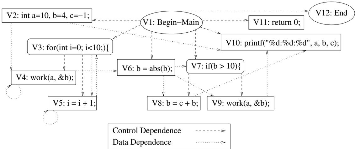
**Figure 2.3:** PDG for CFG in Figure 2.2
