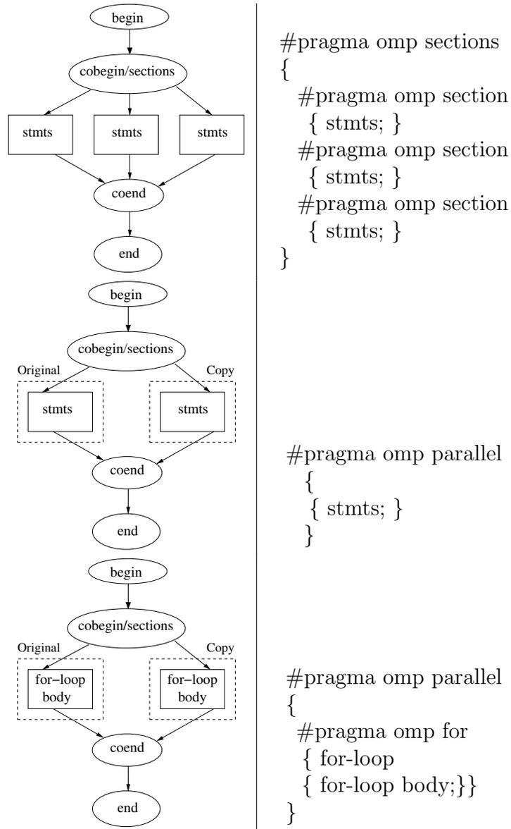
**Figure 3.1:** OpenMP (a)Sections (b)Parallel (c)For Modeled as Cobegin/Coend
