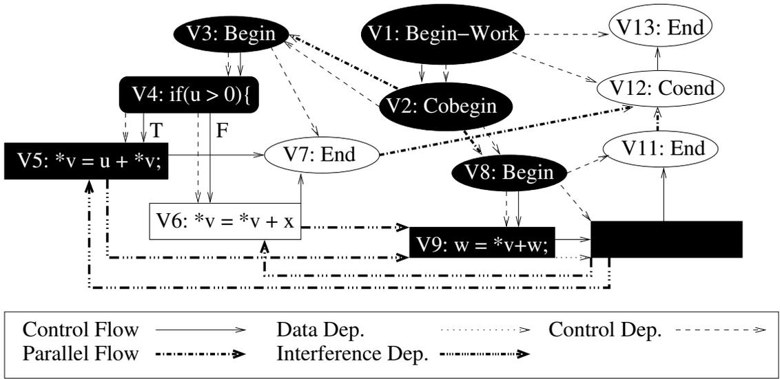
**Figure 3.6:** Threaded Intraprocedural Slicing Example
