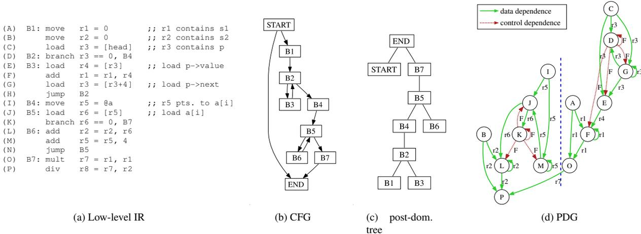
**Figure 2.** For the example in Figure 1: (a) low-level IR, (b) CFG, (c) post-dominance tree, and (d) PDG.
